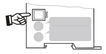
Only a ROPEX comunication interface is allowed to be connected to the diagnostic interface. Connecting another device (e.g. a telephone cable) could result in malfunctions or damage to the controller.
