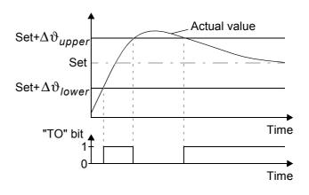
Unlike the "Temperature reached" status bit ("TE" bit), the actual temperature is evaluated independently of the control mode.
