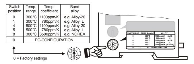
The settings for a temperature coefficient of 780ppm (switch position 1 and 5) are only available on controllers manufactured as of October 2003.
