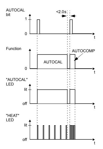
The "HEAT" LED blinks repeatedly when the "AUTOCOMP" function is executed and the actual value output (terminals 17+14) is set to 0...3°C (i.e. app. 0 VDC).
