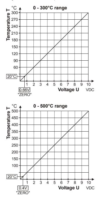
An indicating instrument can be connected to this output in order to visualize the temperature of the heatsealing band.
