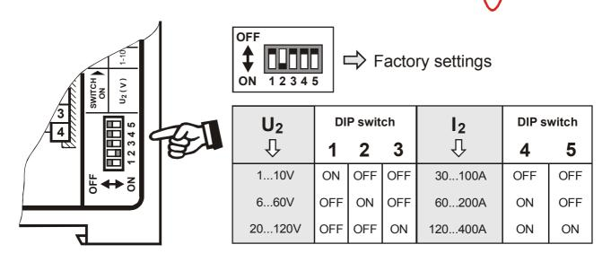
If the secondary current I<sub>2</sub> is less than 30A, the PEX-W2 or PEX-W3 current transformer must have two turns ( $\$  ROPEX Application Report).
