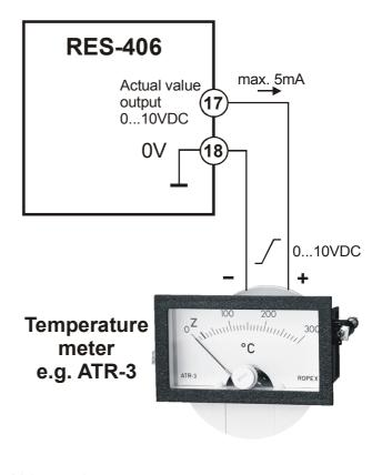
Voltage values: 0VDC → 0°C 10VDC → 300°C or 500°C (depending on the controller configuration)
