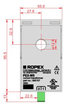
The current transformer is mounted on a top hat rail (TS35) measuring 35 x 7.5 mm or 35 x 15 mm in accordance with DIN EN 50022.
